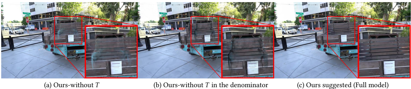
Fig. 8. Gains using the transmittance term T to eliminate "ghosting" effects with our 3DSMoES regression. We compare gating functions (a) without T ( 3DSMoES-T_{n,d} ), (b) with T in denominator ( 3DSMoES-T_n ), against (c) T in both nominator and denominator (full model, our suggested variant). The suggested solution effectively eliminates ghosting.
